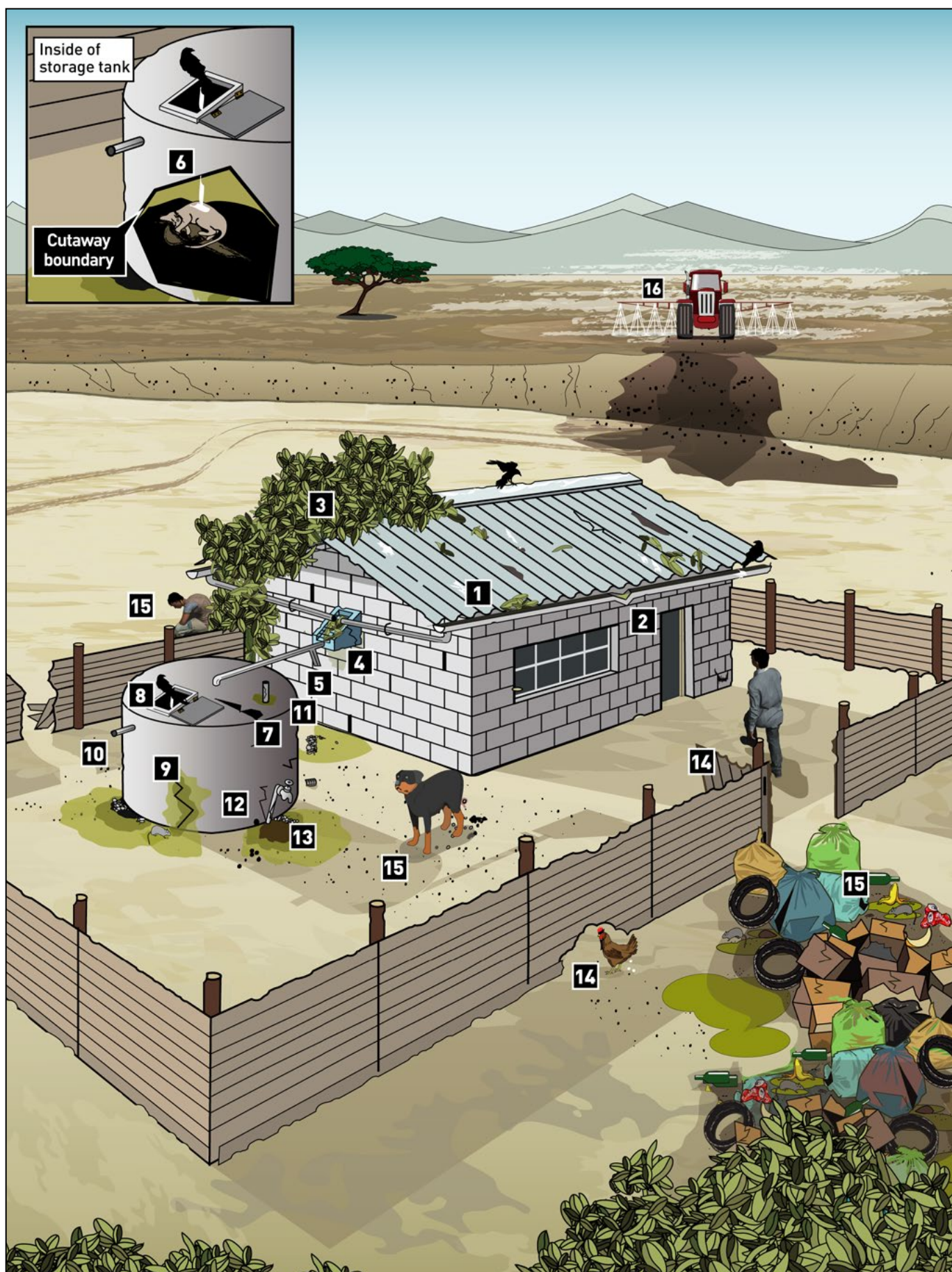
Figure 1. Typical risk factors associated with a rainwater collection system
