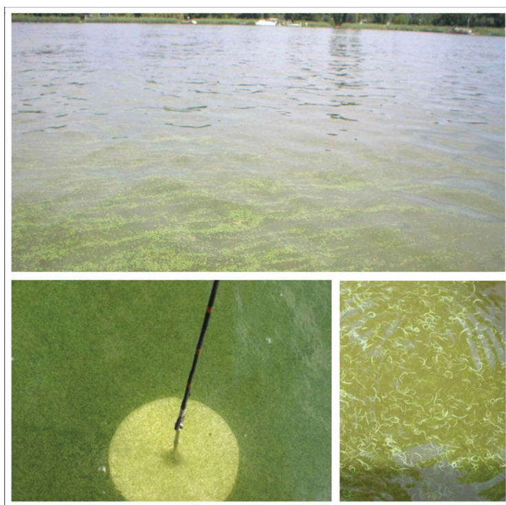
Figure 5.6 Streaks, specs and Secchi disc reading depicting Alert Level I conditions.
