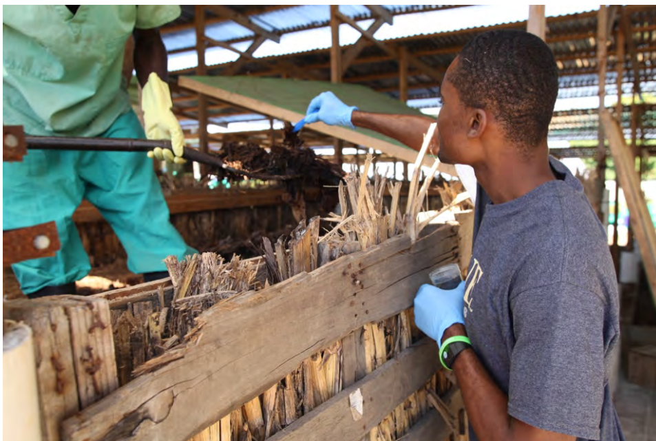
Figure 22: sampling a pile to test for pathogens
