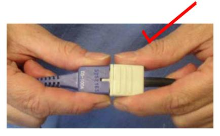
If the cable is pulled, small wires inside will break
