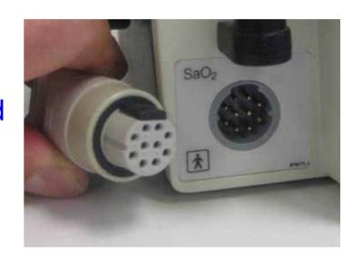
When disconnecting and connecting probe, grip the plug firmly and not the cable.
