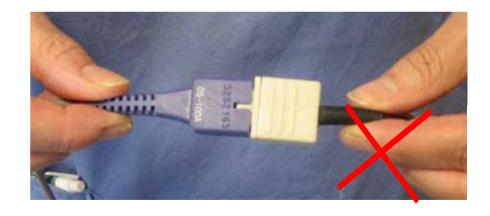
When disconnecting and connecting probe, grip the plug firmly and not the cable.
