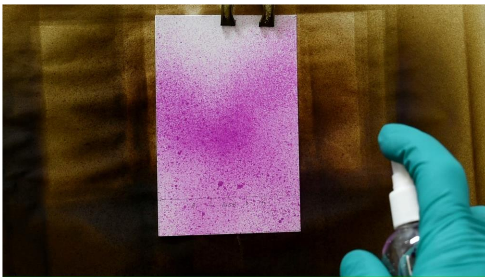
Image 1. Spray the developed plate with the visualization solution using an atomizer.
