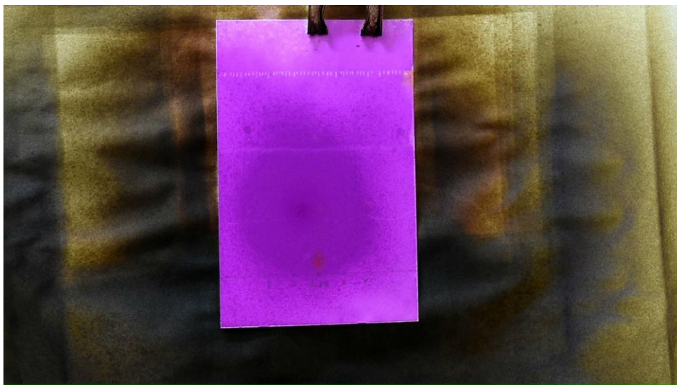
Image 2. Spray the plate with the visualization solution until a fully covered purple background is obtained.
